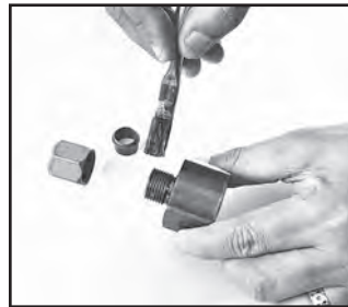
Step 1 – Lubricate thread and cone of Ferulset Tool (or fitting body).
