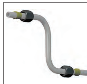
Fig. R30— Nuts and sleeves assembled before flaring
