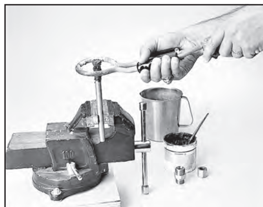
Fig. R22 – Multi-flame torch brazing
