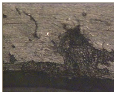
Pitting on filter end-cap
